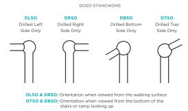
When required stanchions can be drilled one side only on both the top and intermediate rails or only on the top or intermediate rail. Drilled one side only stanchions need to be nominated at the time of ordering along with the correct nomination in which you require.
